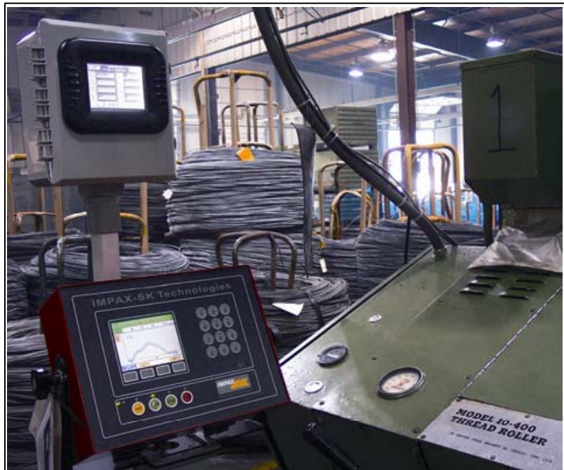
IMPAX TSS System for Downtime Analysis & Production Monitoring (top) working with an IMPAX SK force monitor (bottom)—installed on thread rolling machine at an ITW plant in Oconomowoc, WI, USA.
